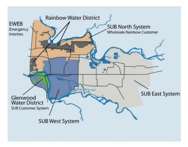
Rainbow is connected to Springfield Utility Board (SUB) and Eugene Water and Electric Board (EWEB), allowing each utility to provide some assistance to the others in the event of a regional emergency. SUB and EWEB are supplied from a combination of groundwater and surface water sources. Rainbow relies on groundwater alone for our normal water supply, although one well is subject to influence from the McKenzie River so it is classified and treated as surface water.
